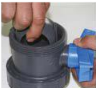
Ball is held with fingers on both edges and removed. Here, ball can be pushed on the bottom to support the removing force.
