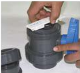
Ring is opened by turning counter clockwise.
