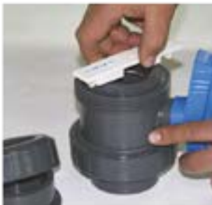
Ring is opened by turning counter clockwise.
