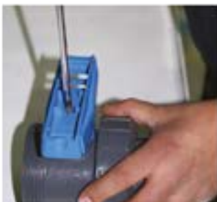
The screw on the handle is removed with a screwdriver.
