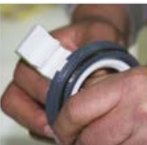
Ball inside bush is taken out by hand together with its seal ring.
