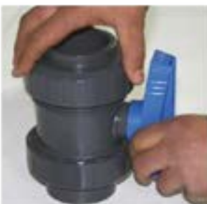
The union nut on the bush side is turned clockwise and removed. Union nut and pipe connection is removed.
